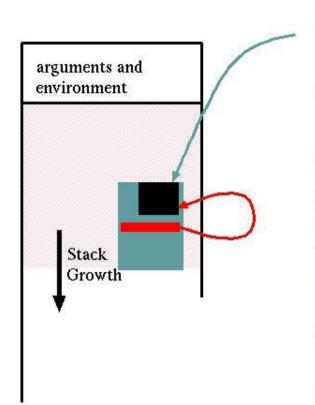
Attacker overflows buffer on stack Note: Buffer is ALWAYS at the same place
